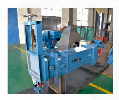
The sealing structure of the warehouse bottom unloading device can be divided into two forms: soft sealing and rigid sealing. The soft sealing structure uses wool felt to seal between the valve core and the valve body.
